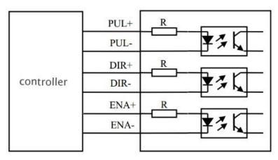
common anode wiring
